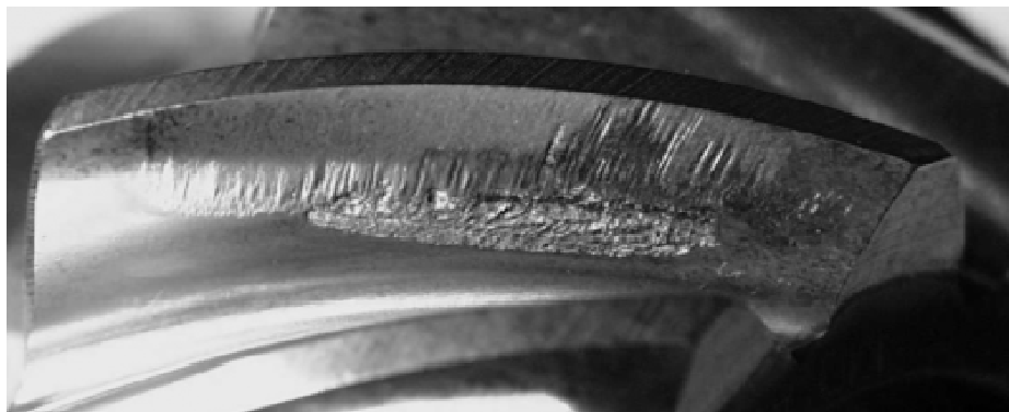
Figure A4: NASA Spiral Bevel Gear Rig Gear Damage.
