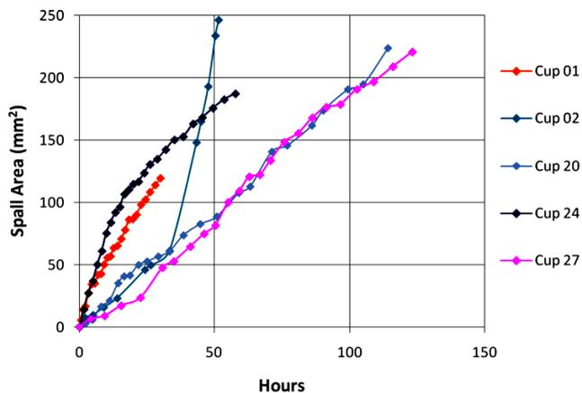
**Figure 6: Spalling on cups during spall-propagation tests.**
