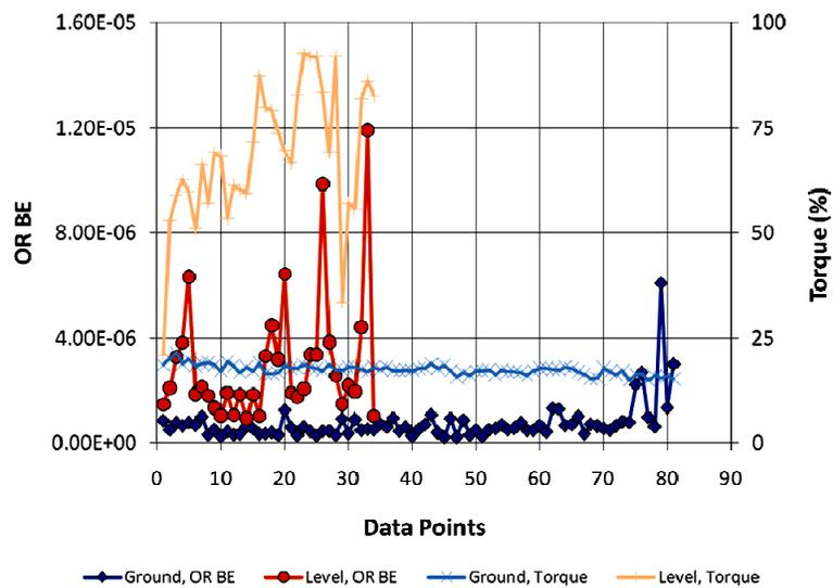
Figure 15: Bearing energies and engine torque for different flight regimes.
