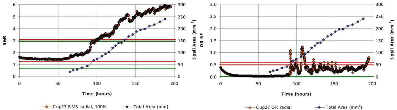
**Figure 11: Cup27 RMS, OR BE and Spall Area Growth.**
