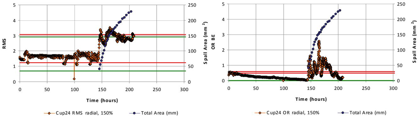
**Figure 9: Cup24 RMS, OR BE and Spall Area Growth.**
