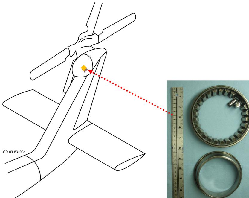
**Figure 2: Location of accelerometers to monitor TGB output shaft thrust bearing.**
