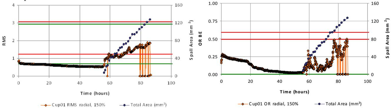
**Figure 7: Cup01 RMS, OR BE and Spall Area Growth.**
