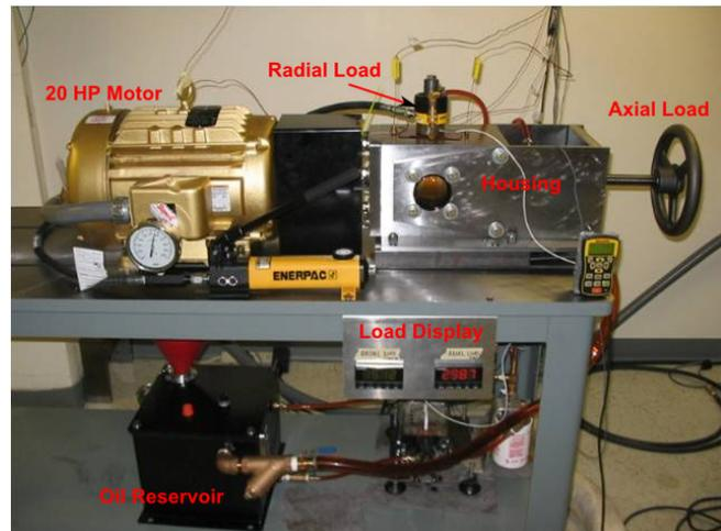
Figure 4: Spall-propagation test rig for TGB bearings.
