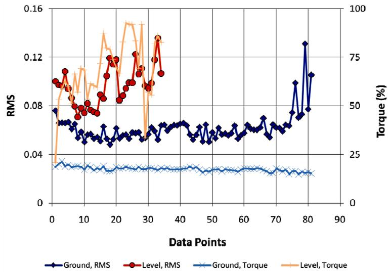
Figure 14: RMS and engine torque for different flight regimes.
