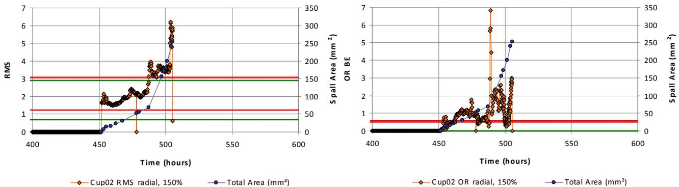
**Figure 8: Cup02 RMS, OR BE and Spall Area Growth.**
