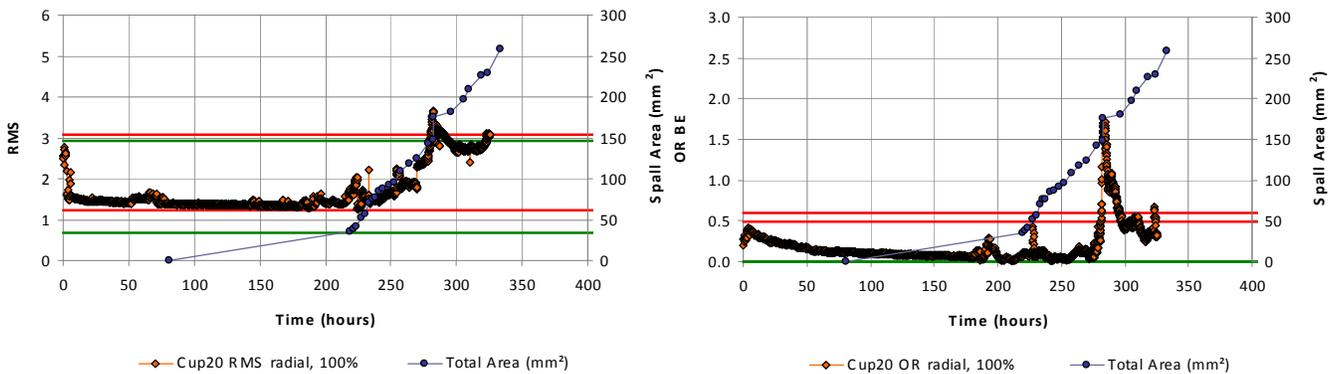
**Figure 10: Cup20 RMS, OR BE and Spall Area Growth.**
