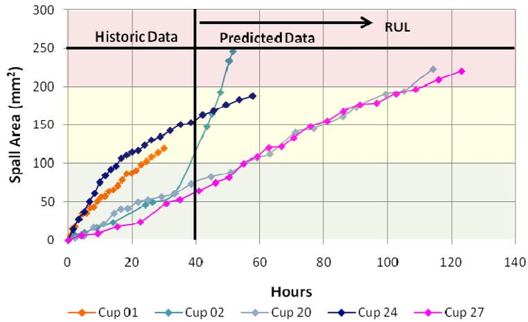
Figure 13: Spall growth rate on cups.
