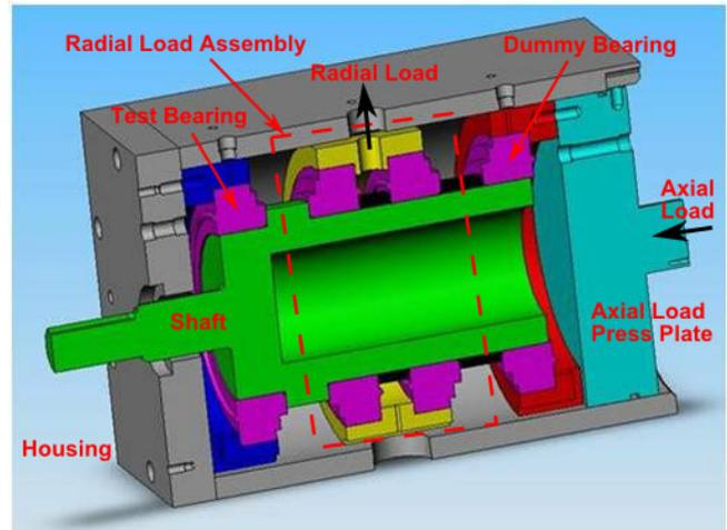
Figure 3: Cross-section of test rig housing.
