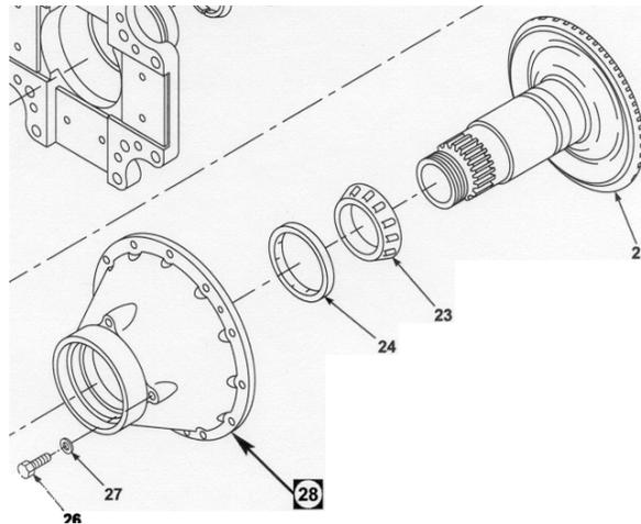
**Figure 1: Assembly drawing of TGB bearing cup and cone (Ref. 2).**
