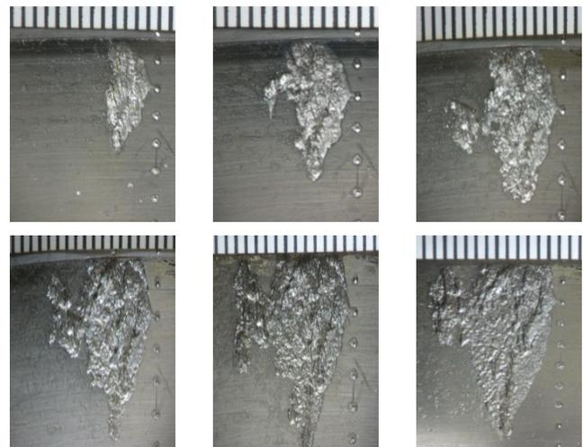
Figure 5: Example of spall propagation photos.
