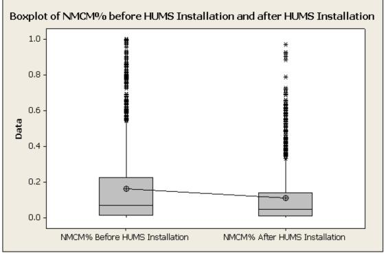
In the above plot, the 5.3% reduction in NMCM rates from before to after installation can be readily seen.
