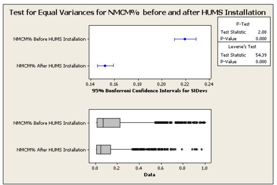
The above plot reveals the test for Equal Variances for Group A (before DSC/HUMS installation) and Group B (after DSC/HUMS installation).
